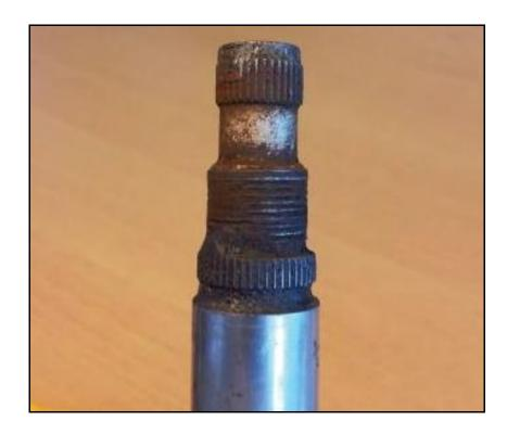
**Photo No. 2**: Example of corrosion found on NLG torque link apex pin following fleet inspection
