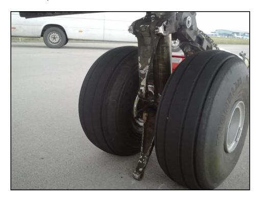
**Photo No. 1**: Separated Torque Links
