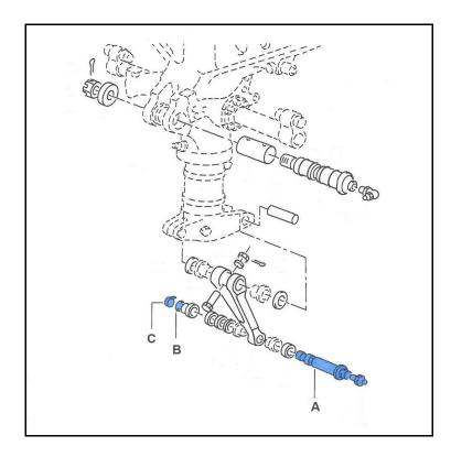
**Figure No. 2**: Detail showing torque link apex pin (A), retaining nut (B) and serrated (locking) washer (C).
