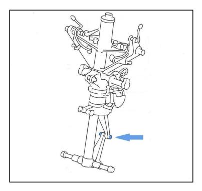
Figure No. 1: Location of torque link apex pin on nose leg assembly
